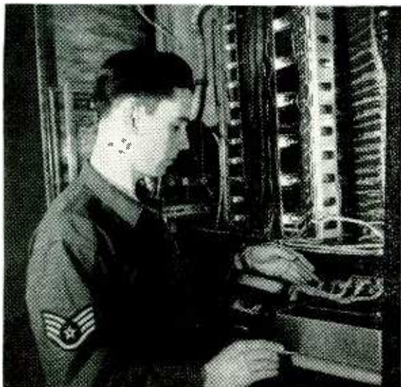
Checking the circuits of the vacuum-tube trainer.
